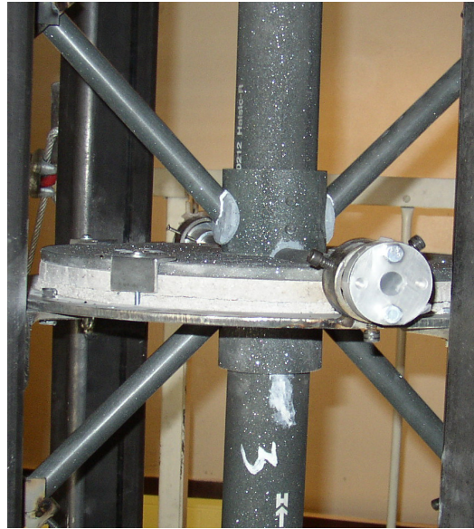
Figure 24 Window section with optical accesses in three orthogonal directions - the insulation was not been placed yet
